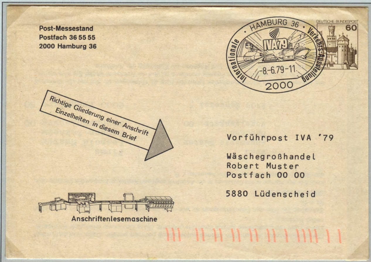
Printed to order (Germany) from Hamburg to Lüdenscheid: code representing 0885 9, left to right code reading. Value 9 points to internal tray or city area. Code gaps represent the value eg: llxx = 4+7 = 0 ; lxllx = 7+1 = 8
