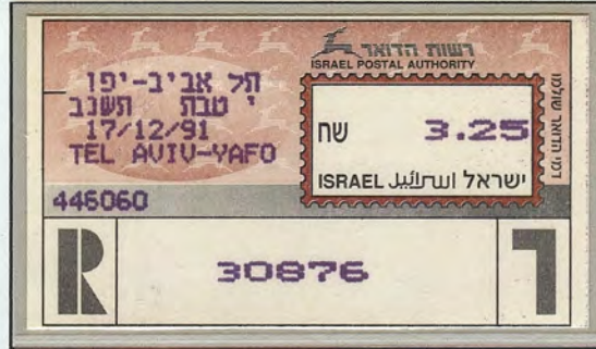
▲ pre-printed registered label (Israel): text printed with a 9-needle dot-matrix printer using purple ribbon.
