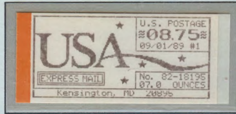
Thermal transfer print used at the 'Autopost' experiment, a self-service postage vending machine. The stamp is printed at selling time. Tests have taken place in the congressional post office in Washington, D.C. and Kensington. After a lot of problems the experiment was cancelled.
