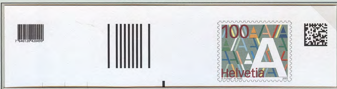
Stationery (Switzerland) with 3 types of bars; EAN-13 (left), 2-Dimensional CP-code (right) and sorting bar code (center)
